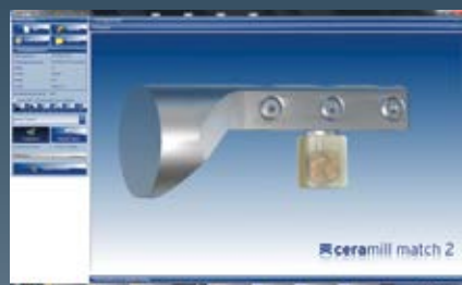
Processing of VITABLOCS TriLux forte with rendered representation of the shade gradient
